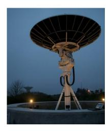
The 3.8 metre dish owned by Satellite Applications Catapult is being loaned to the project to track the ISS and will ensure real time video will be available during the schools' contacts scheduled for early next year. The dish is almost in the shadow of the 29 metre dish "Arthur" built in 1962 to receive the first transatlantic television signals from the Telstar-1 spacecraft.
